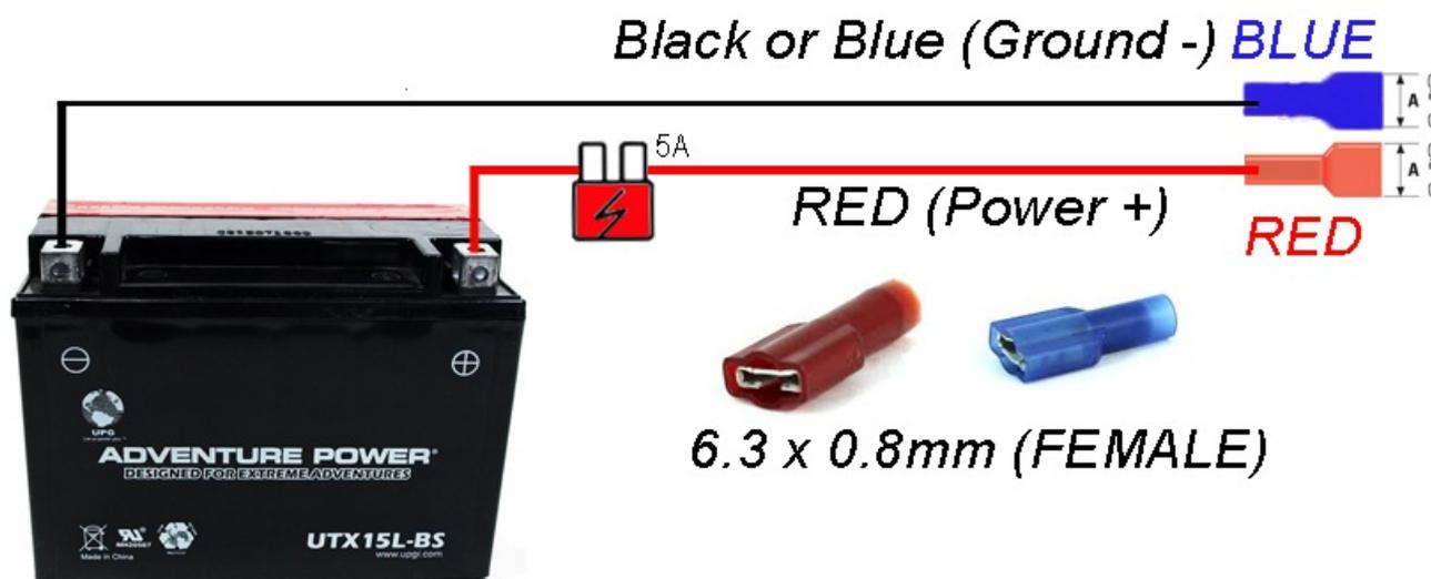
**FLEXIBLE CABLE** -  $2 \times 1.5 \text{mm}^3$  (square millimeter)
